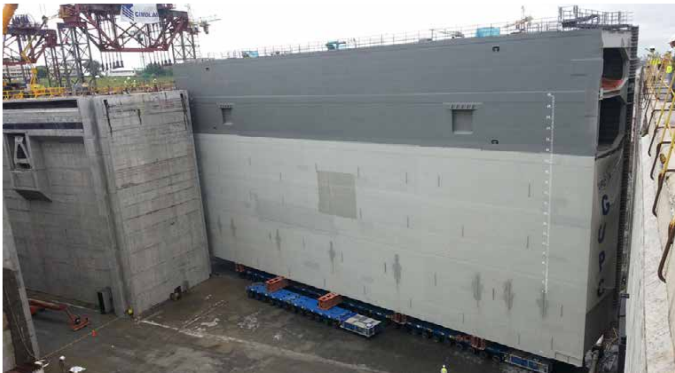
SPMT - MSPE EVO 2 type - more than 160 axes available - 9,500 t total load capacity
