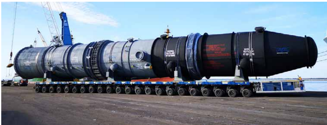
SPMT - MSPE EVO 2 type - more than 160 axes available - 9,500 t total load capacity
