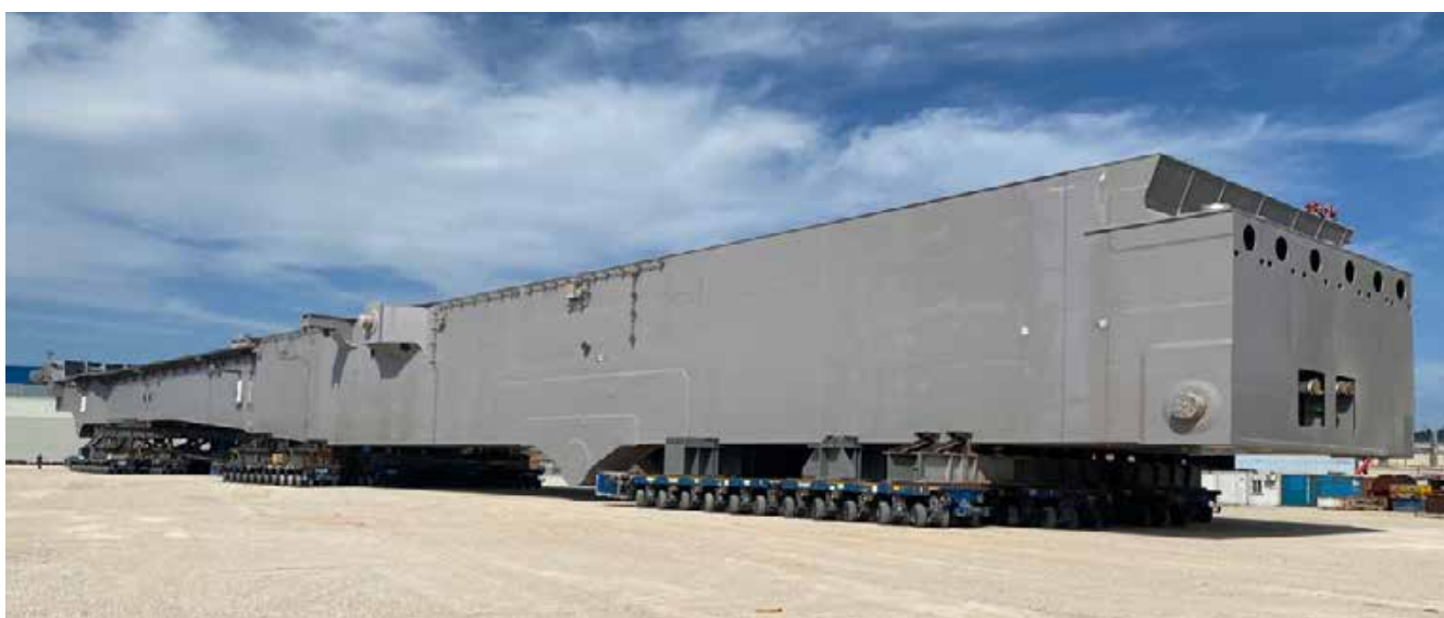
SPMT - MSPE EVO 2 type - more than 160 axes available - 9,500 t total load capacity
