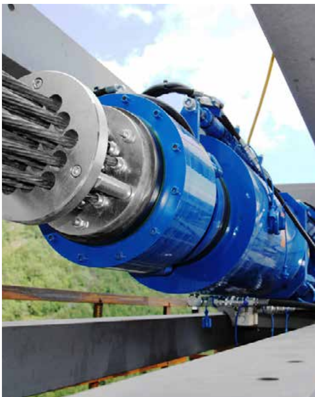
STRAND JACKS - HSL 2000 type - 12,000 t lifting cap.
